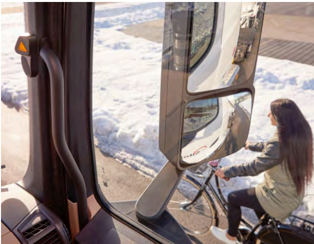
If there is immediate danger of collision, the assistant will warn the driver
