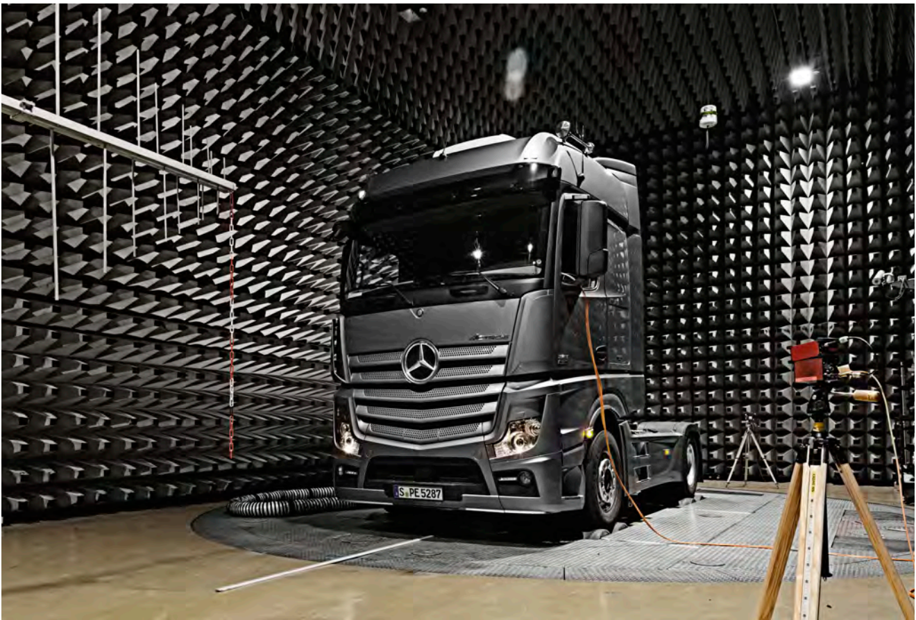
EMC test in a laboratory that is especially shielded against external electromagnetic interferences.
